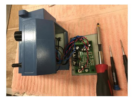
3. Locate the trimmer potentiometer on the control board as shown below.
